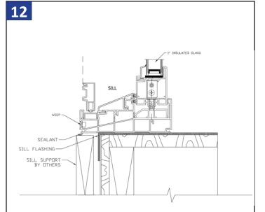
Attach a sill support block beneath the sill. Apply a bead of sealant at the nose of the sill and support block. Make sure sealant doesn't block the bottom sill weep hole covers.
