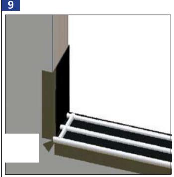
Apply three 3/8" continuous beads of sealant across the entire width of the rough opening sill. Apply a 3/8"continuous bead of silicone  $\frac{1}{2}"$  from each side of the rough opening. The bead will run the entire depth of the jamb starting at the face of the wall.
