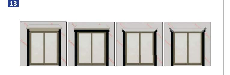
Cut and apply side flashing. Side flashing should run from the bottom of the sill flashing to 4" above the rough opening. Cut and apply head flashing. The head flashing should run slightly past the edge of the side flashing as shown. Flip down the top flap of the house wrap. Tape the cut seams of the house wrap.
