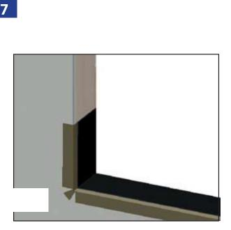
Flashing tape must cover the entire sill. If needed, apply an additional flashing piece over the first one (start from the exterior and work towards the interior). Maintain a minimum 1"overlap.
