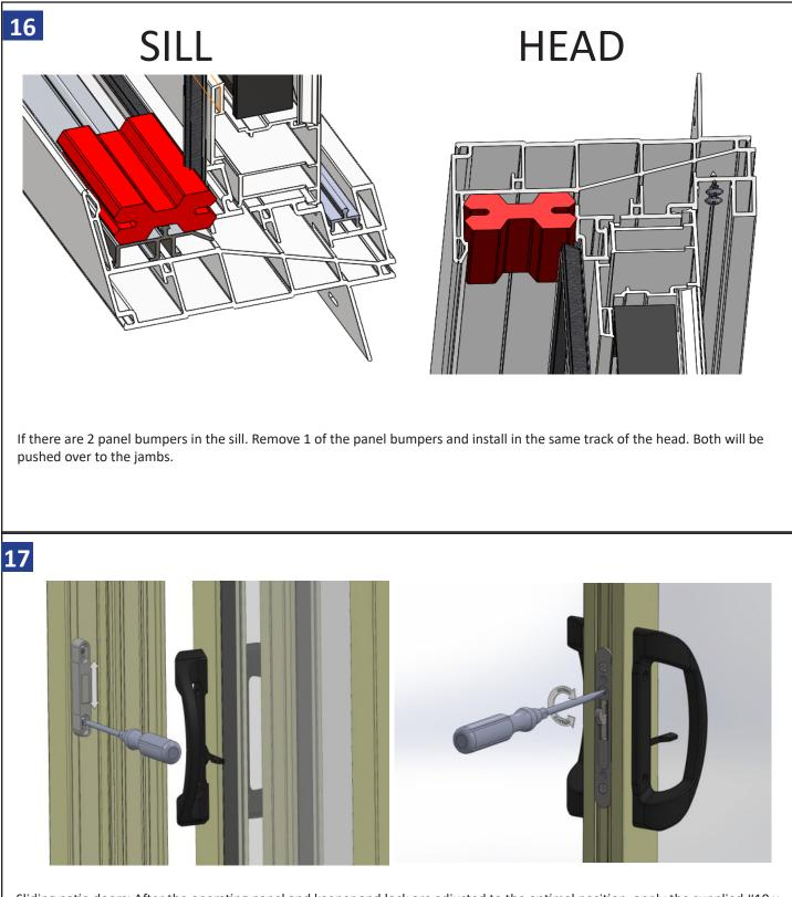
Sliding patio doors: After the operating panel and keeper and lock are adjusted to the optimal position, apply the supplied #10 x 1 %" screws through the top and bottom holes of the keeper. Pre-drill the holes using a 1/8" bit prior to assembly.
