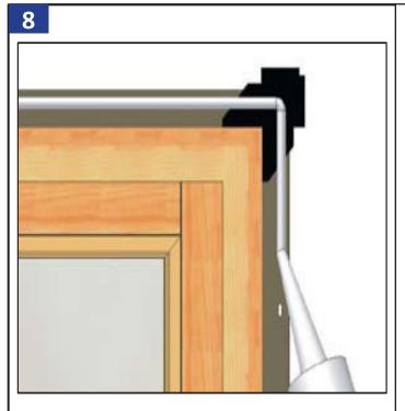
Apply a continuous 3/8" diameter bead of sealant along the backside of the nailing flange. Bead must run around both sides and across the head, in line with and completely covering the nail flange holes.
