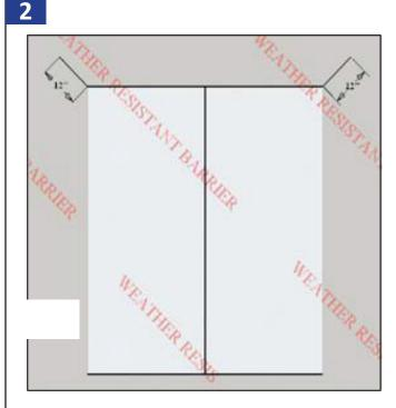
Apply the house wrap according to the manufacturer's instructions and cut T-pattern opening as shown. Cut top flap angles at 45 degrees and 1" longer than the width of the flashing tape being used.
