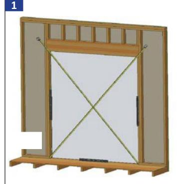
Measure and verify the opening is sized correctly. The rough opening should be a minimum 1/2" (but not to exceed 1") wider and taller than the unit. Check that the opening is square. The diagonal measurements need to be within 1/8" of each other. Verify the rough opening is plumb and level. The sill must be level for proper unit operation.
